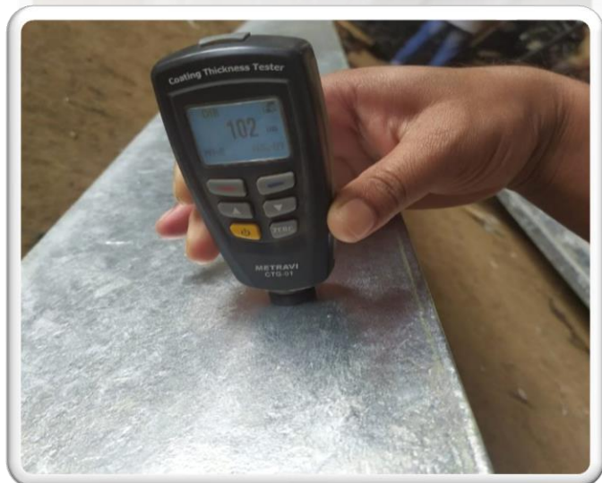
Inspection of 20 mm fabricated Galvanized Steel Angle
