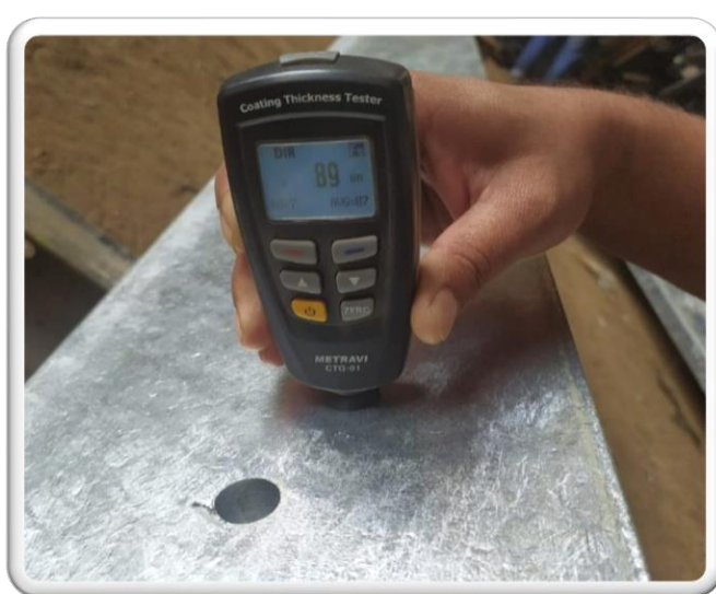
Inspection of 12mm fabricated Galvanized Angle
